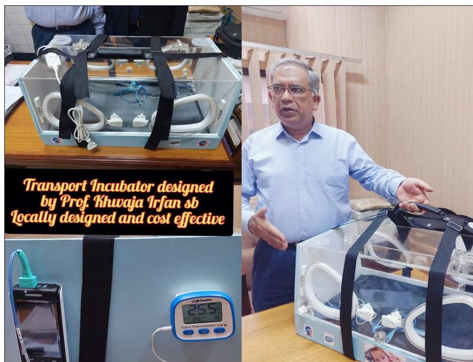
Figure 1: Prof. Irfan Waheed Khawaja introducing a locally made neonatal transport system with in-built temperature monitoring and management system, and pulse oximeter.
